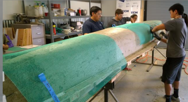
Figure 14: Placing Reinforcement Mesh
